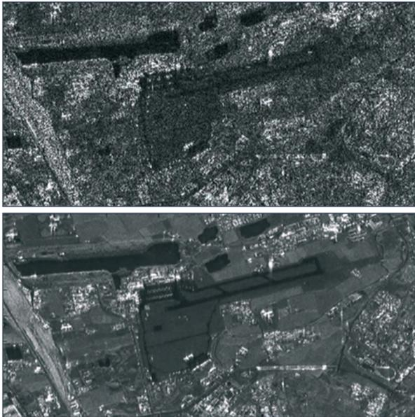
**Figure 2.** Speckle noise reduction using temporal multilooking (illustration from Ferreti *et al.*, 2007)
